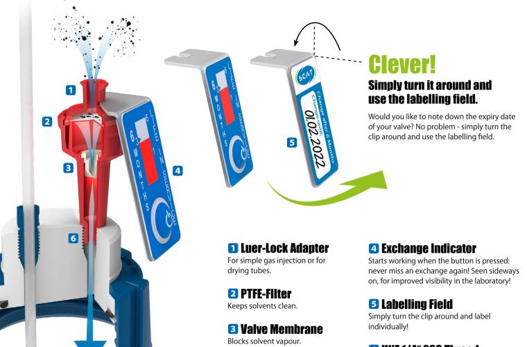
Integrated check valve prevents the evaporation of solvents.
