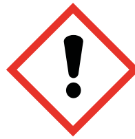
GHS 07 Health hazard/ Hazardous to the ozone layer
