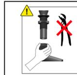
**Tighten the screw fittings of the connection pipes only hand-tight! Do not use pliers or other tools with high power transmission!**
